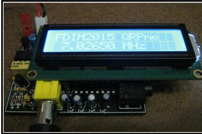
I like the Sparkfun LCD modules. I use a white on black display (5 volt version) with built in white backlight.
