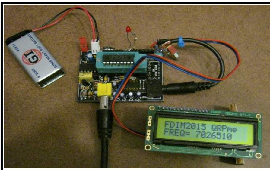
I also use the serial backpack version (at times) which requires TTL level signals, so a jumper plug is installed at U3. The display requires +5v, ground and signal. The crazy wiring above picks up the +5v and ground from the last 2 pins of the LCD connector which normally powers the LCD backlight and sends it out to power the backpack electronics and display.
