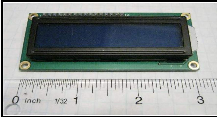
A COMPATIBLE LCD SCREEN IS ABOUT 3" LONG AND USES THE KS0066U OR EQUIVALENT HITACHI CONTROLLER. IT HAS A 16 PIN INLINE MALE HEADER FOR PLUGGING INTO THE PCB. I USED A GDM1602K LCD MODULE FROM SPARKFUN.
