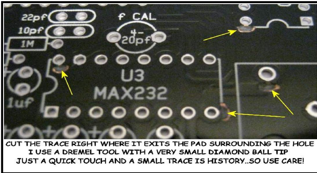
The first pair of trace cuts are on the TOP side of the circuit board where the +5 volt power trace leaves the MAX232 chip, on Pin 16 and enters the OSC CAN socket on Pin 14. From the picture above, you can see the grind marks where I ground off the small trace just as it exits the actual solder pad.
